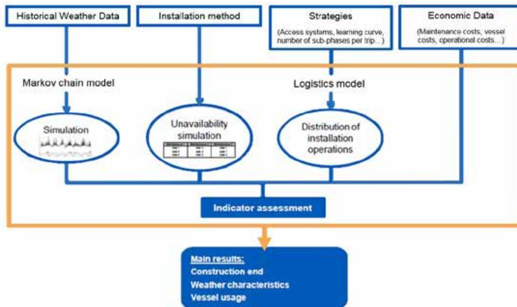
Figure 1: Model Inputs and Architecture of the ECUME I
